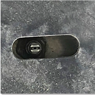
Sixteen 25°, size 15 nozzles spaced 6-inches apart, for low undercarriages
