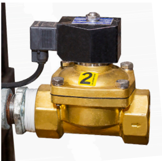
Auto flow control solenoid that opens water flow valve when system is on and closes when off to prevent drainage
